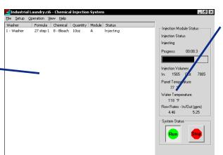
Injection module status shows you what the injection module is currently doing - including flow rates and temperatures.
