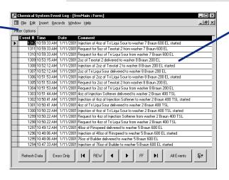
System event log shows you just about everything that's happened on the chemical system - from errors to setup changes to injection starts and completions.
