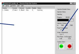
Injection module status shows you what the injection module is currently doing including flow rates and temperatures.
