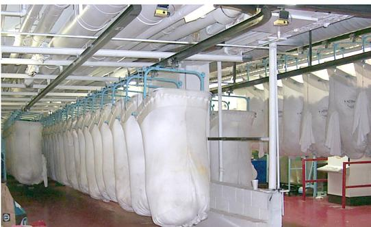
Slings wait to be loaded into open-pocket washer/extractors on a CCS automated rail system.
